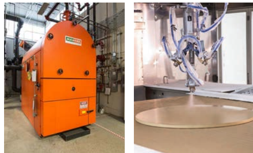
Left, a biomass furnace burns waste and heats the factory; right, a robotic finish system, the first of its kind in the country, provides not only superior finish quality and consistency for clients, but reduced over spray and closed chamber system for employee and environmental wellness.
