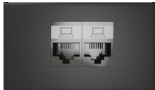
2 RJ45s (data/network connectors)
